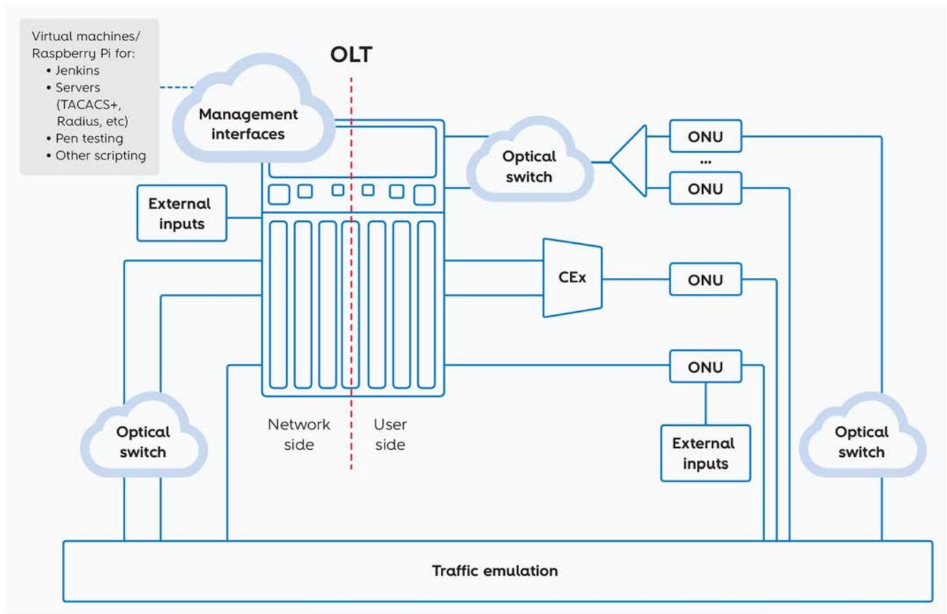
**FIGURE 5** – OLT test automation scenario
