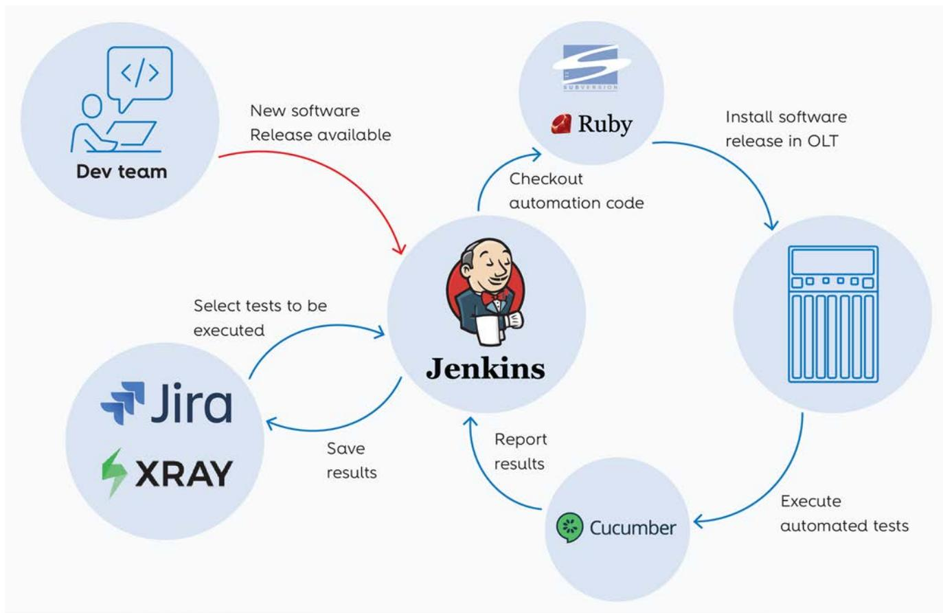
FIGURE 4 – OLT test automation process
