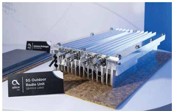
**FIGURE 1** – Standard casing solution with embedded antennas
