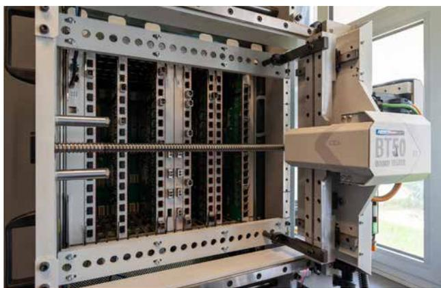
**FIGURE 8** – Automated test equipment used for physical insertion and removal of OLT cards
