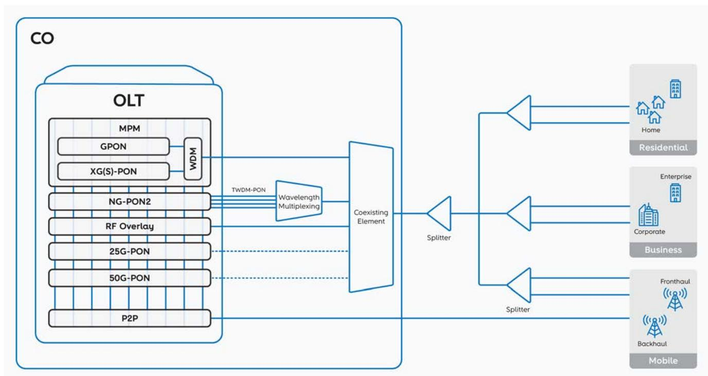
**FIGURE 1** – Coexistence scenario, G-PON, XG(S)-PON and HSP (CO – Central Office)
