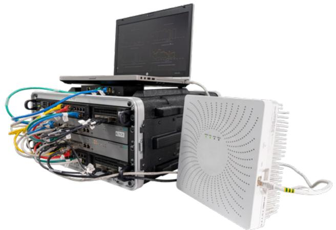
**Figure 6** - 5G ‘in-a-box’ used kit
