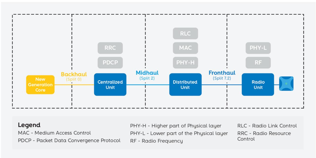
**Figure 8** – Splitting points and functional components of Altice Labs’ 5G solution
