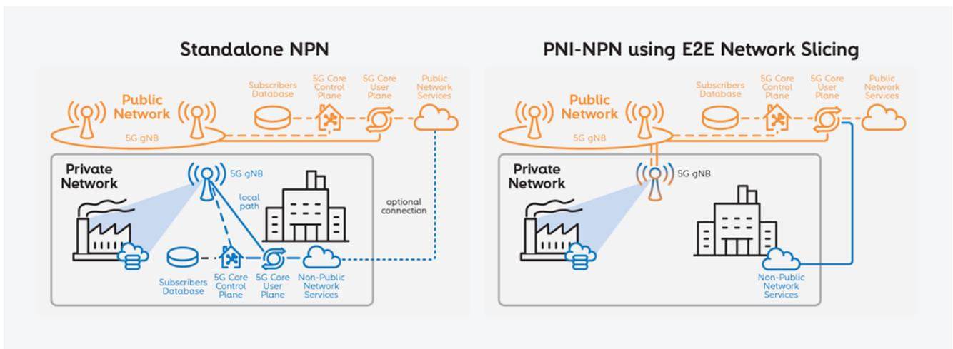
**Figure 1** – NPN deployment flavors (5G-ACIA)
