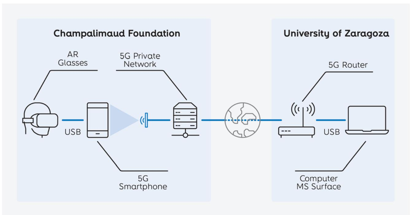
**Figure 7** - End-to-end diagram used to setup the demo
