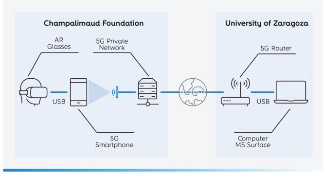
Figure 7 - End-to-end diagram used to setup the demo
