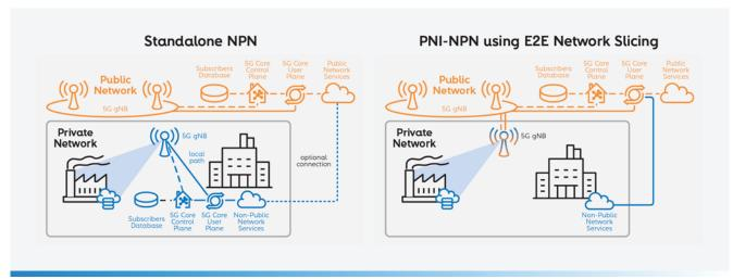
Figure 1 - NPN deployment flavors (5G-ACIA)
