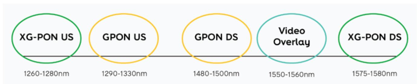
**FIGURE 1** – Wavelength plan for GPON, XG-PON, and video overlay
