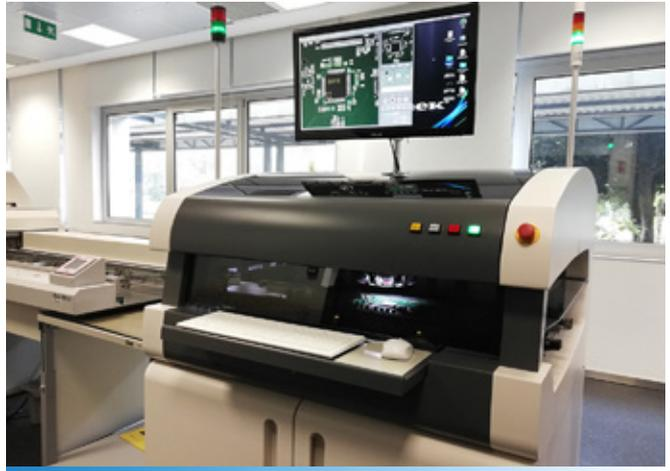
**Figure 4** - Automatic optical inspection
