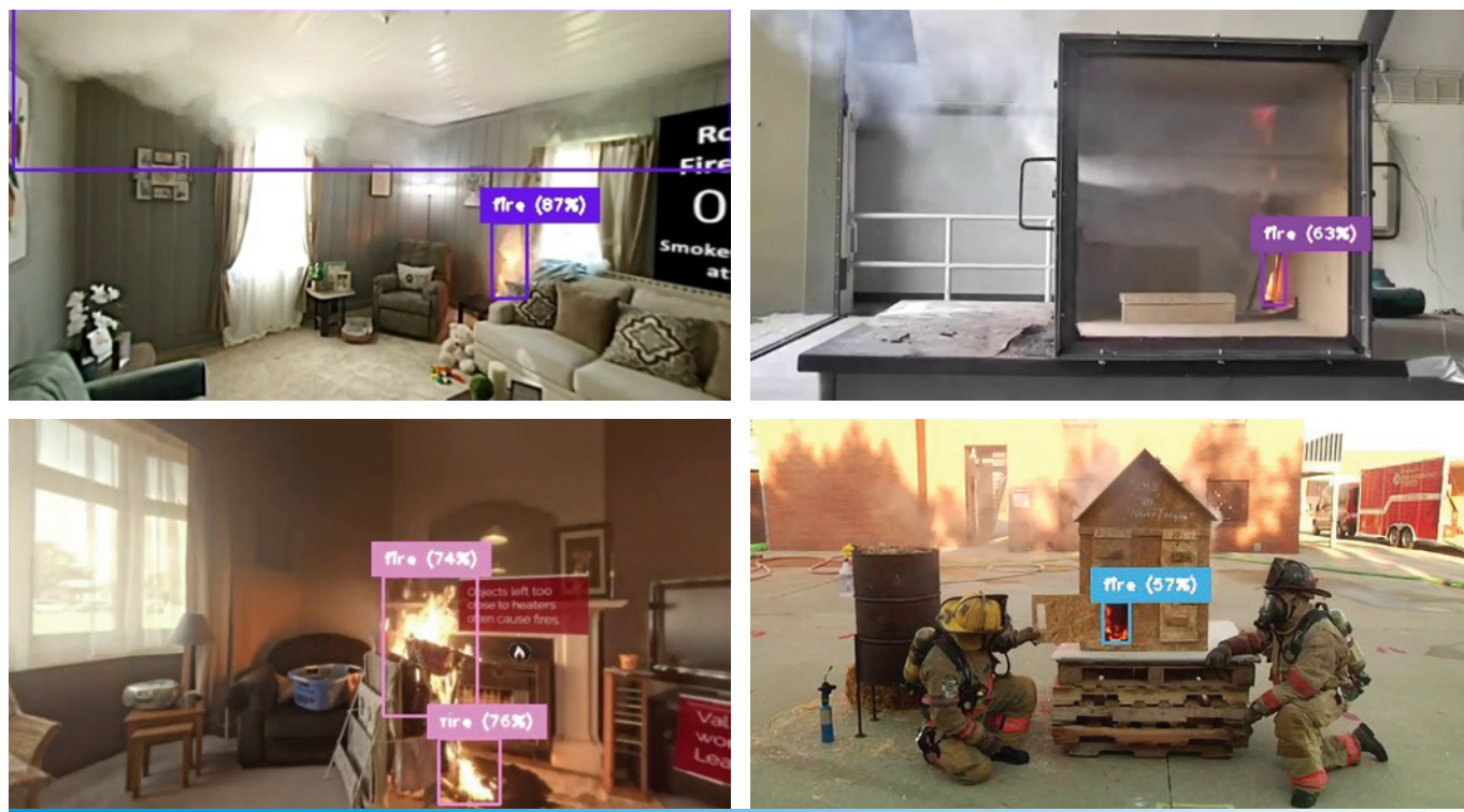
FIGURE 7 – Accuracy of the best model (model #10) for the four tests 7
