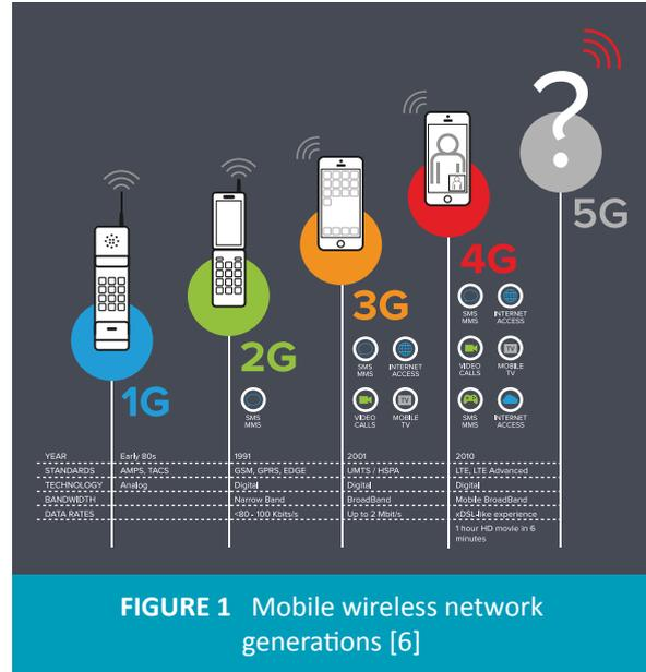
FIGURE 1 Mobile wireless network generations [6]
