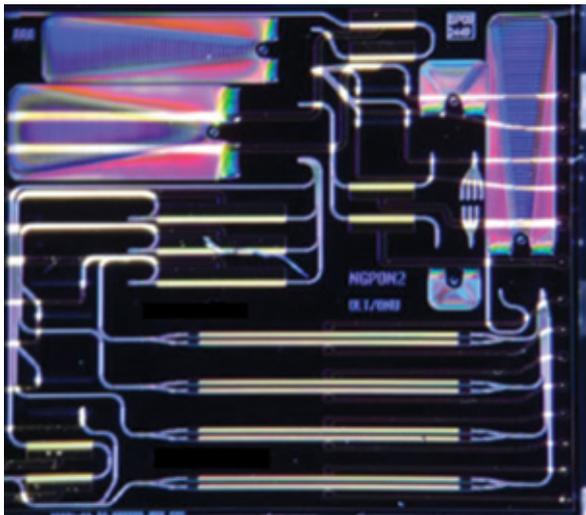
**FIGURE 9** PIC for NG-PON2. Chip received from the foundry
