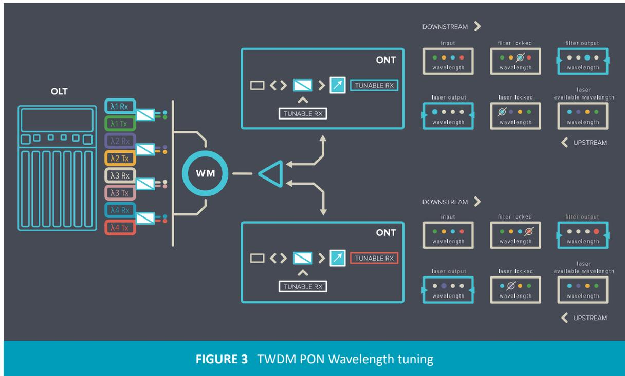
FIGURE 3 TWDM PON Wavelength tuning
