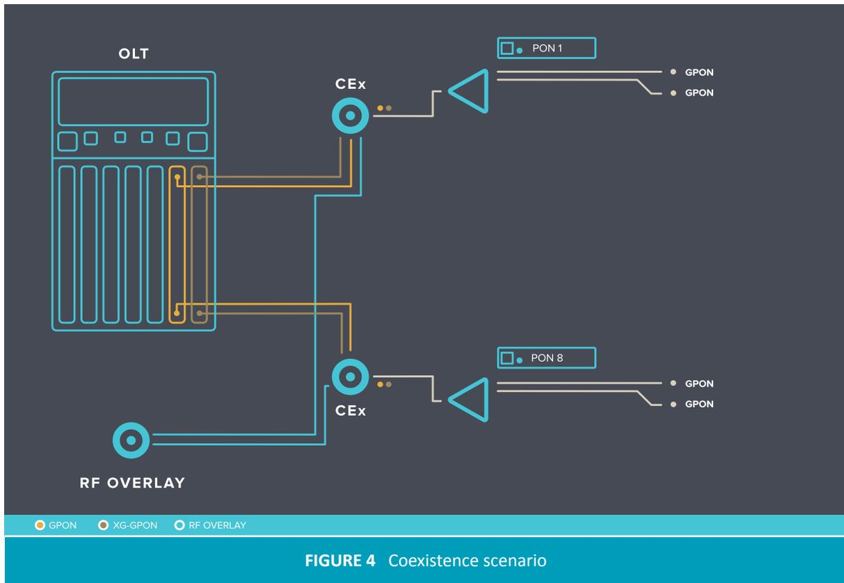
In order to coexist with legacy PON networks a coexistence element is needed. This coexistence element can have different configurations depending on the technology that the service provider wants to deliver (Figure 4).
